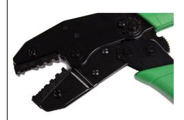
SMA, SMB, SMC, RATCHET CRIMP TOOL - Our tool frame is made from top quality hardened Steel for long life use, it features a ratchet controlled cycle mechanism to ensure a correct crimp every time and is fitted with a precision manufactured die set to crimp coaxial connectors with very small diameter cables RG174, 178, 179, 180 and 187.
